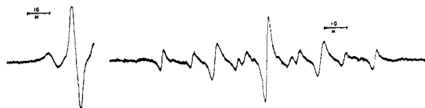
Figure 2. First derivative of the esr spectrum of p -benzosemiquinone-1- 13 C ion in DME with potassium as counterion at room temperature. On the left of the main spectrum is shown under high modulation the end proton line on the high-field side together with the 13 C satellite.
